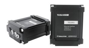
TE1001 is a point-to-point converter tool from 100Base-T1 Automotive Ethernet to 100Base-TX ordinary Ethernet. We provide matching cable with D-SUB9 Automotive Ethernet interface and RJ-45 crystal head interface, which is convenient to connect ECU to PC with Automotive Ethernet interface.
