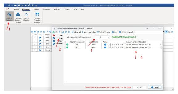
In the hardware configuration, the CAN / CAN FD protocol can be switched, and the baud rate and switch terminal resistance can be adjusted. After the configuration is completed, click application can take effect.
