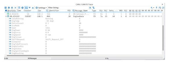
Solution: display in a fixed display or time order, expand or fold the signal display, and filter the string, click the following icon to operate:
