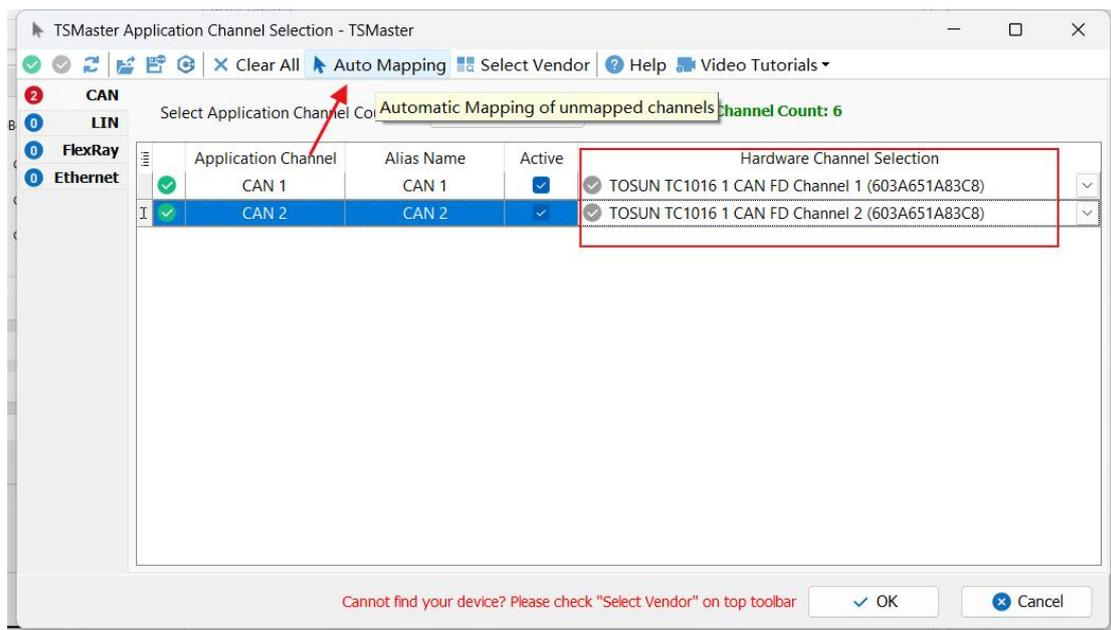
If the channel is selected correctly, it is necessary to ensure consistent port communication between the two channels, as shown in the figure below:
