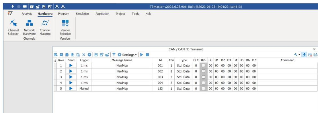
After the hardware connection is completed and the software is configured, the function of message sending can be realized:
