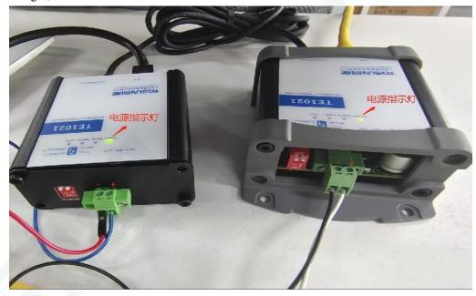
Step 2: Device RJ 45 network port is connected to ECU through the network cable; Ethernet interface is connected to ECU through the cable, as shown below:
