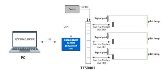
For bus communication analysis board cards, such as TTS1018, TTS1026P, and TTS1034, simply insert the board cards into the slots of the TTS0001 (in some cases, the TTS0001 needs to be powered), and the board cards can be used by connecting the corresponding USB interface of the TTS0001 to a computer.
