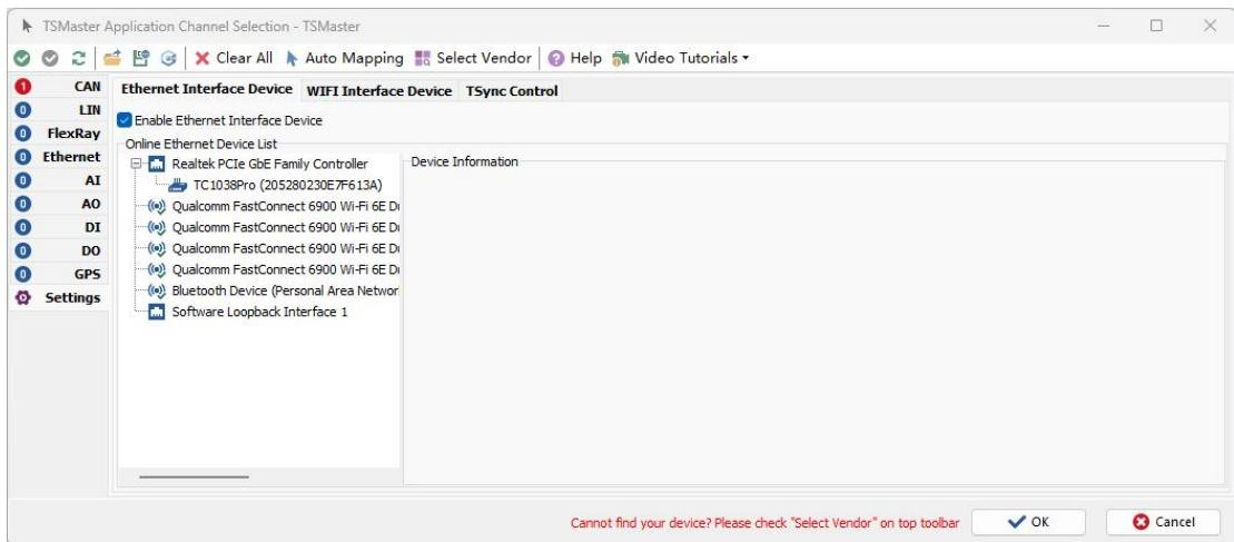
In the "Channel Selection" interface, select the type of bus technology in the left sidebar and configure the application channel count.
