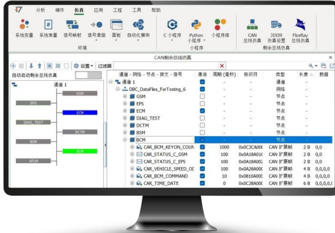
With the TSMaster software, it is possible to achieve multiple buses simulation such as CAN and LIN. ECU code simulation can also be achieved through Desktop HIL (hardware-in-the-loop) features. The Panel feature built into TSMaster allows bus signals association in the panel to achieve graphical display.
