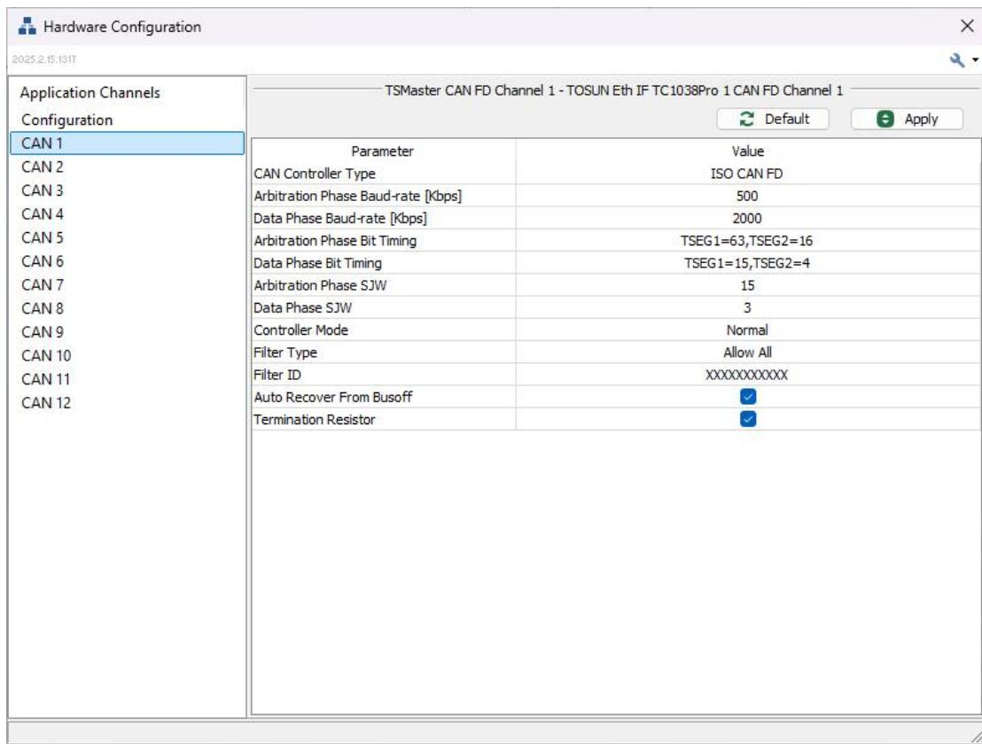
After the configuration, click Analysis->Start and connect the hardware to efficiently carry out works such as bus development, testing, ECU production line, etc. with the powerful TSMaster software. For more detailed instructions on using the TSMaster software, please refer to the TSMaster software manual and the quick start guide.
