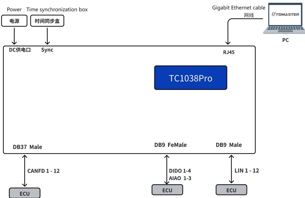
Power the TC1038 Pro via the power adapter interface or Phoenix terminal interface with DC 12V, and connect the device's RJ45 Ethernet port to the PC. Based on users' requirements, connect the corresponding CAN/CAN FD, LIN, DIDO, and AIAO interfaces to the ECU. The TC1038 Pro can then be controlled via the TSMaster software on the PC to communicate with the ECU.
