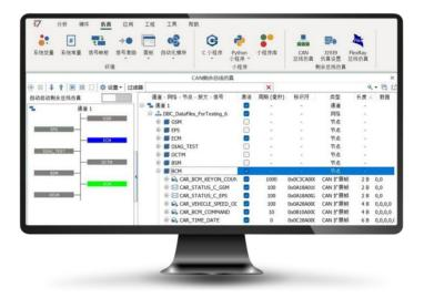
With the TSMaster software, it is possible to achieve multiple buses simulation such as CAN, LIN, and FlexRay. ECU code simulation can also be achieved through soft HIL. The Panel feature built into TSMaster allows bus signals association in the panel to achieve graphical display.
