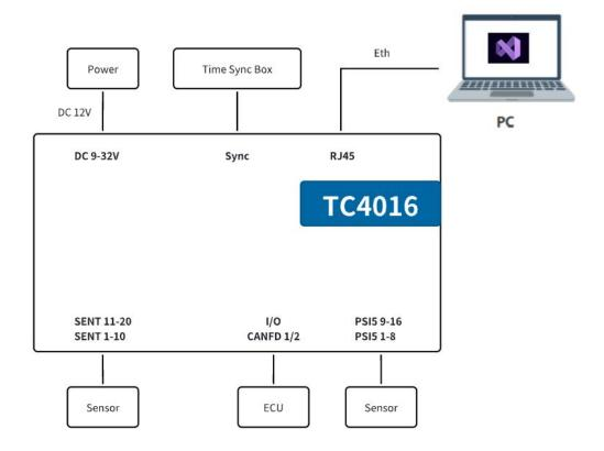
The TC4016 device can be powered via either the DC 12V power adapter interface or the Phoenix terminal block. Connect the RJ45 Ethernet interface of the device to a PC. Depending on application requirements, users can connect corresponding interfaces—SENT, CAN/CAN FD, DIDO, AIAO, and PSI5—to sensors or ECUs. Once connected, the TC4016 can be controlled directly from the PC.
