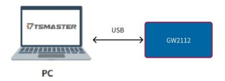
When the users want to perform configuration for the device, simply connect it to a PC via USB. Once the Config light is solid, users can use the TSMaster software for the corresponding configuration functions.
