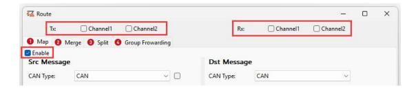
The routing configuration feature comes with built-in routing, so to make the routing configuration effective, the basic routing option in the channel configuration must be turned off. This is because basic routing forwards data without any processing.
