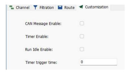
CAN Message Enable: Check "CAN Message Enable" to indicate the activation of an event upon receiving a CAN message.
