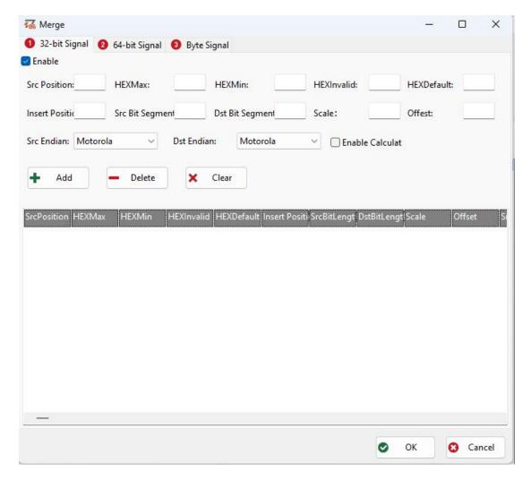
Src Position, Src Bit Segment, Src Endian are used to confirm the source of the data.
