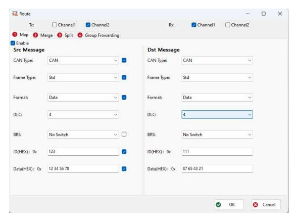
Demo: As shown in the figure below, the source message was sent with an ID of 0x123 and data of 0x12345678. After being converted by the GW2112, it was transformed into a message with an ID of 0x111 and data of 0x87654321.
