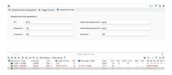
ID: The sample point test form can specify the CAN or CAN FD frame ID for sending
