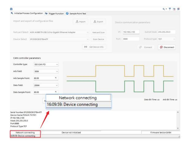
(6) Select the corresponding parameters from "Device CAN Control Parameters", and click "Initialize Device", and the log bar below will display "Initialization Successful".
