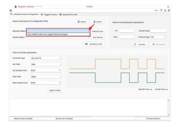
(2) Click "Scan Devices", and after the scanning is successful, the serial number of the disturbance interface (which may include multiple devices) will be obtained in the "Device Selection" drop-down box.
