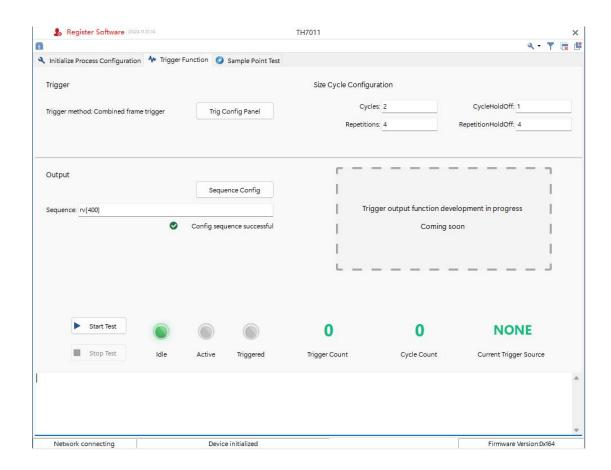
Click "Trigger Configuration Panel" to enter the interference trigger configuration interface.
