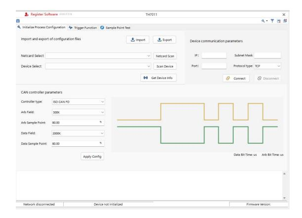
(1) Click "Scan Network Card", and select the network card from the drop-down box after the scanning is successful. If the computer has multiple network cards, you can choose which one to use.
