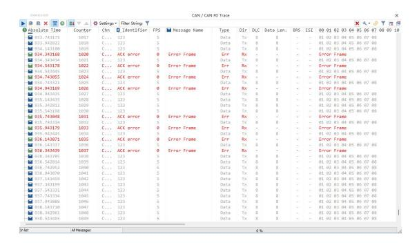
Take a cycle of 2, a cycle interval of 3, a repetition of 4 times, and a repetition interval of 1 as an example, the above figure shows that a total of 8 error frames are generated (cycle \* number of repetitions).
