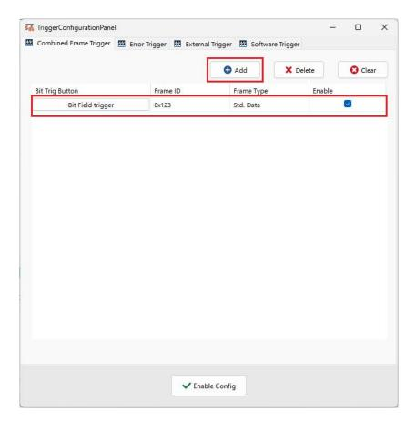
(2) Click the "Bit Field trigger" button to enter the configuration panel, where users can select the bit of Arb field/control field/data field/CRC field for trigger.
