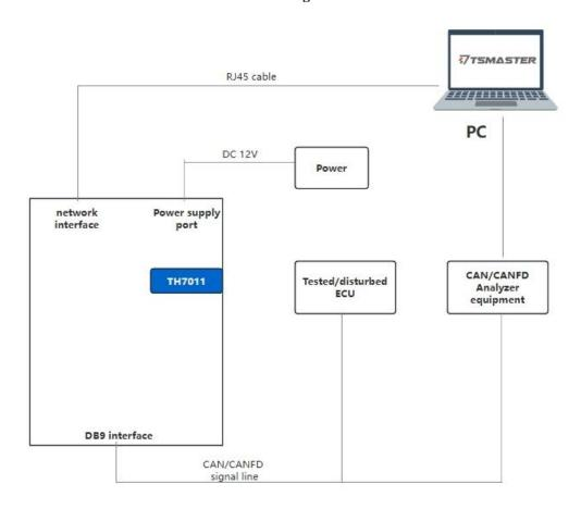
(1) Currently, the disturbance interface cannot monitor messages directly. If you want to monitor CAN/CAN FD messages during interference, as shown in the figure above, you need to connect an additional CAN/CAN FD analyzer device (e.g., TOSUN TC1013 or TC1014) to the bus.
