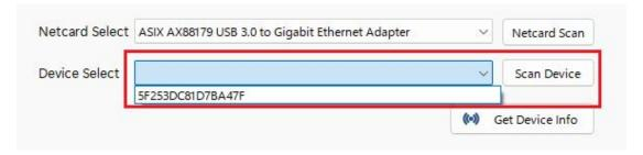
(3) Select a device serial number from the "Device Selection" drop-down box, click the "Get Device Information" button, and the relevant information of the device will be displayed in the parameter column on the right.
