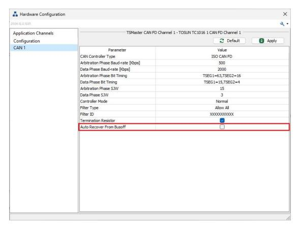
When the TC1016 is set to start message transmission and is subjected to interference using a disturbance interface, it can be observed that after 32 consecutive frames of interference (bit errors), message transmission/reception stops.
