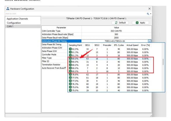
(2) The sampling point of the disturbance interface should be slightly smaller than that of the device under test. For example, if the device under test is set to 80%, the disturbance interface can be set to 75%.
