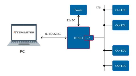
Connect the TH7011 device to a computer via Ethernet, and connect the CAN ECU device to the TH7011. With the powerful TSMaster software on the PC, you can control the TH7011 disturbance interface to perform sampling point testing, disturbance, and other operations on the messages.
