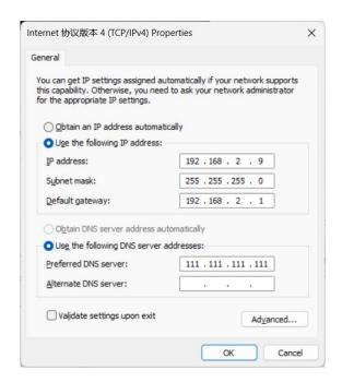
If the computer's network segment is 192.168.2.xx, you can manually change the IP address of the device's communication parameters to be in the same network segment. If the connection to the device fails, check if this is the cause.
