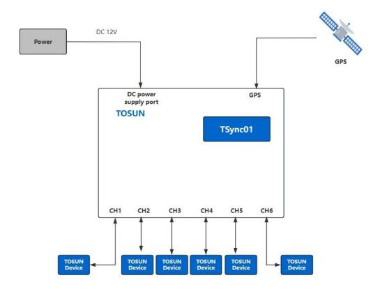
Provide 12V power to the TSync01 device, connect the GPS antenna (for absolute synchronization mode), and connect the devices requiring time synchronization to the TSync01 using LEMO aviation cables to achieve synchronization for up to six slave devices.
