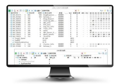
When used with TSMaster software, Tlog1039 supports message transmission/monitoring/playback, bus statistics/logging, and graphical/numerical data analysis.
