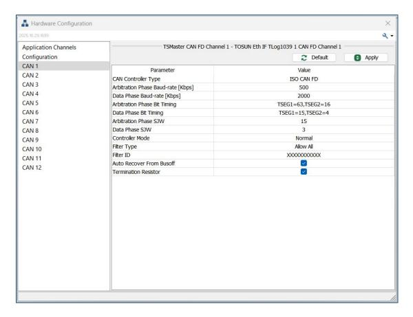
Once configuration is complete, click Analysis->Start to connect the hardware. The Tlog1039, when paired with the TSMaster software, enables efficient development, testing, and production line operations across various automotive bus systems.
