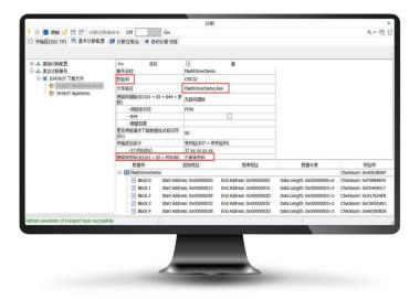
Diagnostics are a key functionality of modern ECUs. During vehicle operation, sensors throughout the system detect various potential faults in electrical and electronic subsystems. TOSUN toolchain supports the development, verification, and UDS-based ECU flashing needed for these diagnostic operations.
