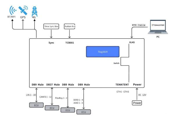
The Tlog1039 is powered through the DC 12V power interface.
