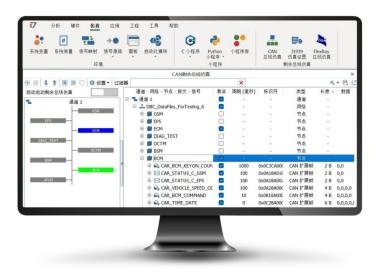
Together with TSMaster software, Tlog1039 enables multi-bus simulation including CAN, LIN, and Automotive Ethernet, as well as code simulation via Desktop HIL (hardware-in-the-loop) features. The built-in Panel function allows graphical visualization of signal data linked to bus channels.
